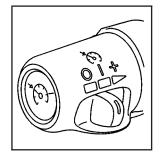
The Adaptive Cruise controls are located on the end of the multifunction lever.
